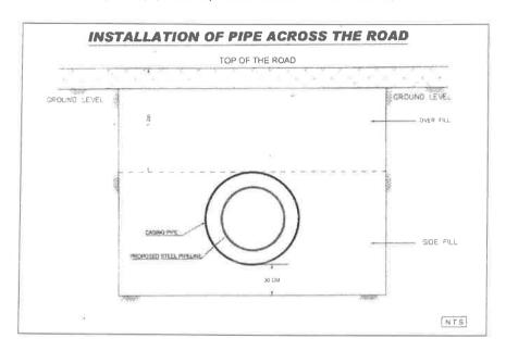
The laying of pipeline across the National Highway / State Highway shall be carried out by Trench Less Technique i.e. either by Boring or Ramming of carrier pipe or by Micro-Tunneling or by Horizontal Directional Drilling without disturbing the normal traffic on the Highway. All the safety measures shall be taken during execution of pipeline laying work across the National Highway/State highway.
